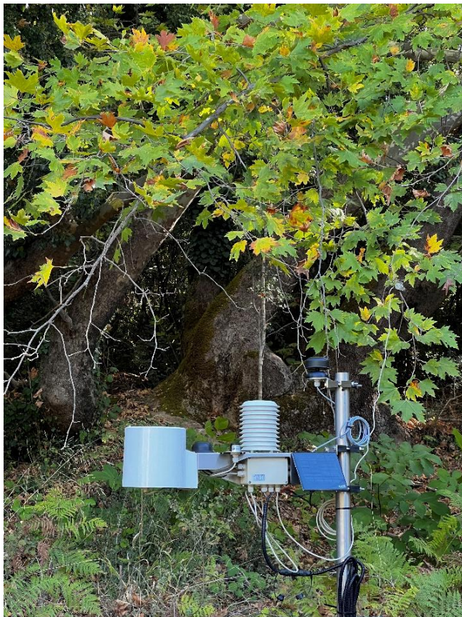
Figure 15. Weather sensor installation in the UCP at Mantoudi-Limni-Agia Anna (Source: AUA)
