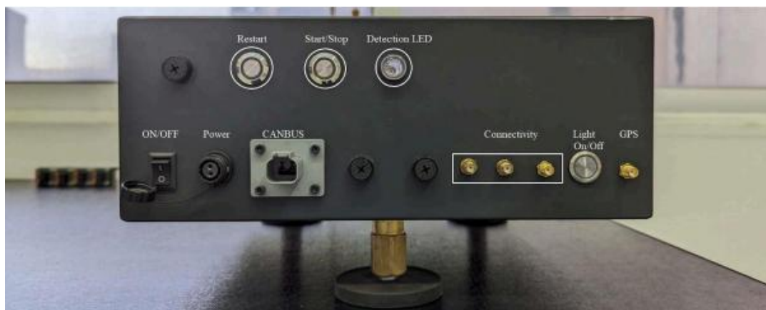
Figure 2. The rear view of the EDEN viewer with the names of the buttons, LEDs, and terminals (Source: EDEN)
