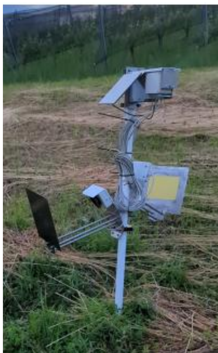
Figure 3. Example of an electronic insect trap installed in the field
